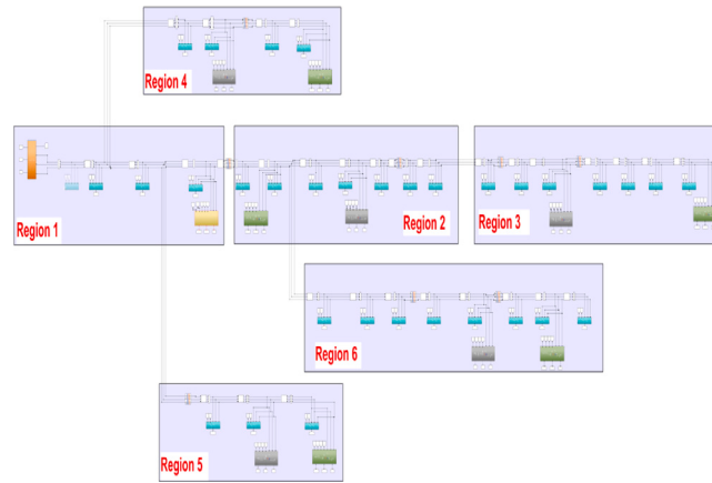
Fig. 10. MATLAB/Simulink model of the IEEE 33 bus system.
